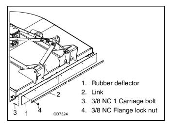
Figure 33. Rubber Deflector Installation
